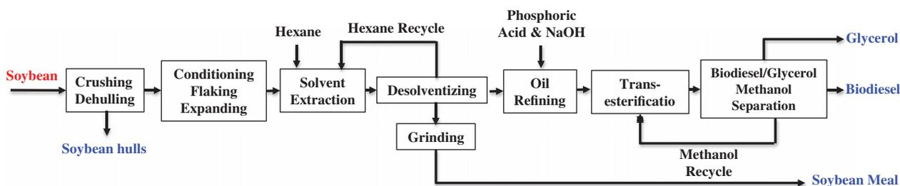
Figure 2. Flow diagram of soybean biodiesel process.
