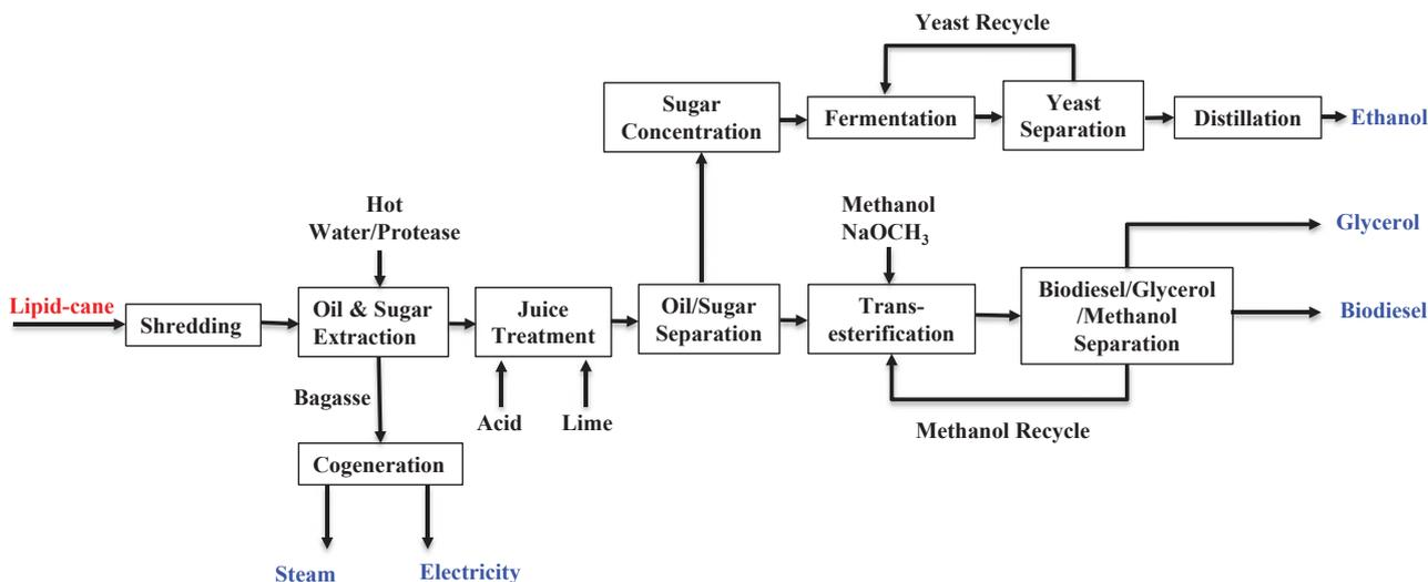
Figure 1. Flow diagram of the lipid-cane process.
